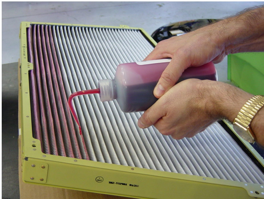
Figure 5: Oiling Filter Media
