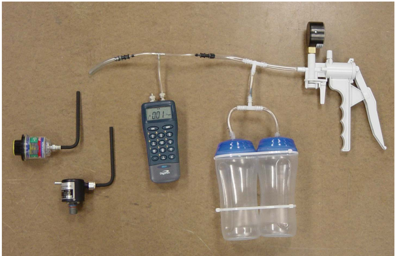
Figure 9: Test Setup with Manometer
