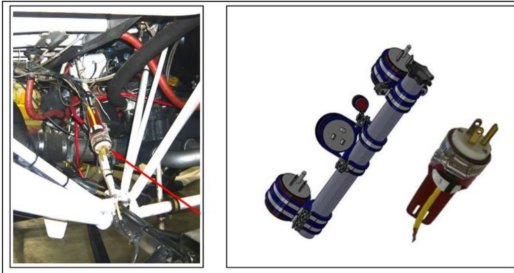
Figure 3 - Examples of plug mounting options: Left - TU01062 circular plug bracket. Right - Plug secured with cushioned clamps, and TU01062 bracket.
