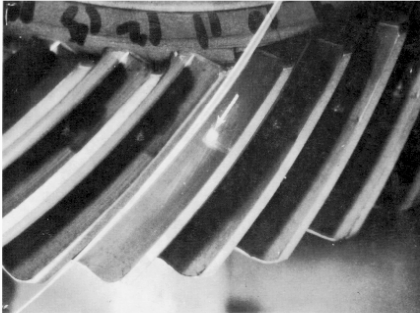
204-040-701 AND 412-040-701 SPIRAL BEVEL GEAR UNACCEPTABLE PATTERN
